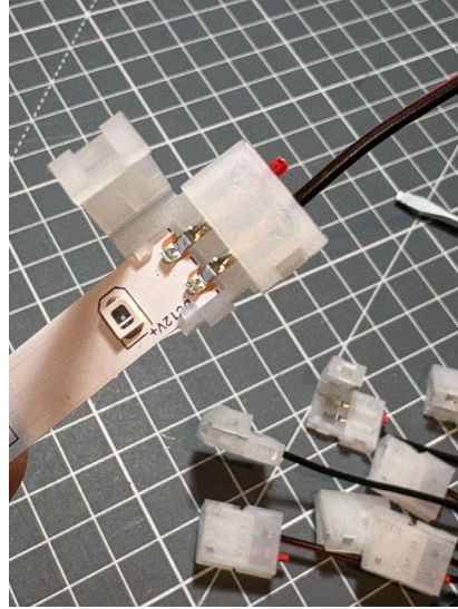
LED strip connected to a pigtail connector before the locking part is clicked into place
