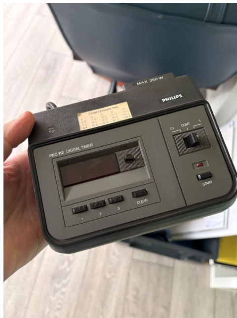
A simple enlarger timer capable of timing 0 to 999s
