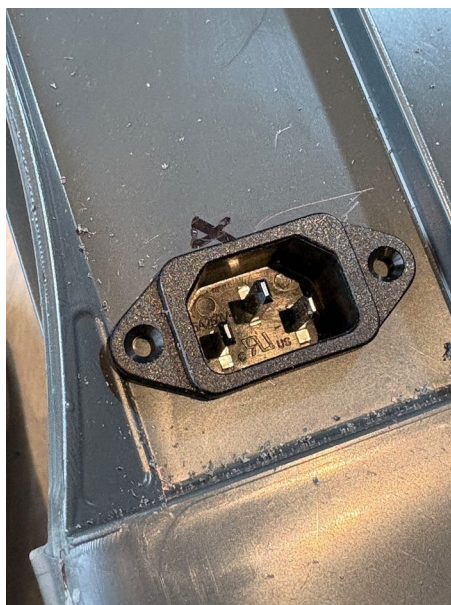
Hole cut for the mains socket; and the socket in place (not yet bolted in)
