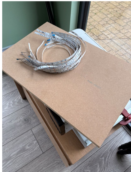
8mm LED strips and 18mm MDF mounting board
